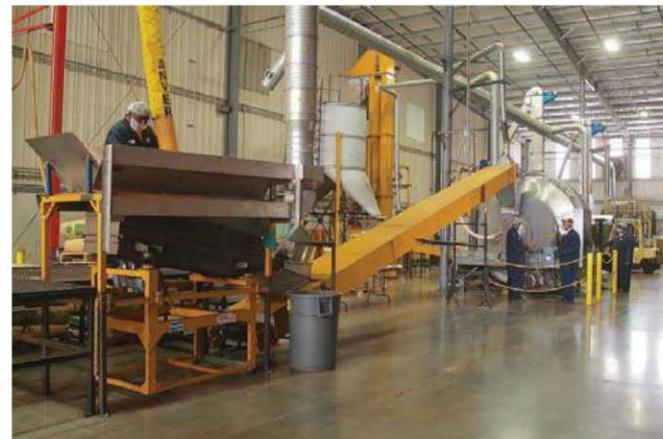
At the warehouse, tea is received from suppliers in sacks weighing between 41 to 64 kg, which are opened by dropping them onto serrated teeth positioned above a vibrating screen, which removes oversized objects. A conveyor, outfitted with magnets to remove any metallic particles, transports the tea into the mixer.
