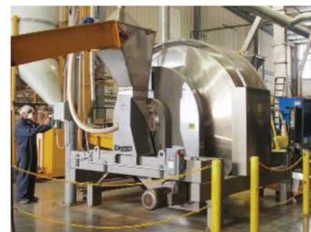
To deliver this consistency, HPT relies on a Munson 3.9 cu m capacity Rotary Batch Mixer.
